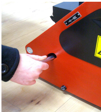
Replacement of the drum -- attention: Lefthand thread !
